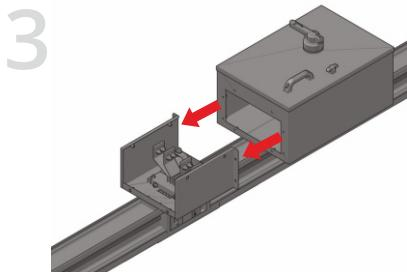
In order to complete the bolt-on installation, place the joint unit onto the busbar and slide it towards the joint.
