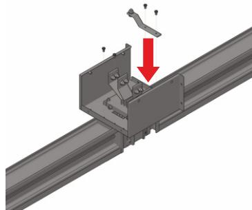
After screwing the bolt-on unit onto the joint, install the earthing conductor as shown in the figure.
