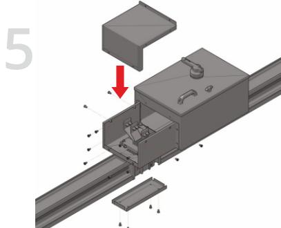
Install the bolt-on cover. Then, connect the busbar joint cover. Screw with M6x12 screws.
