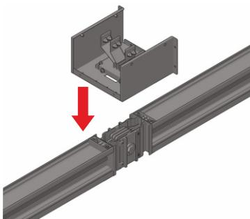
Before screwing the joint of the busbar, align the bolt-on unit with the center of the joint. Then, place the unit and screw the joint block.
