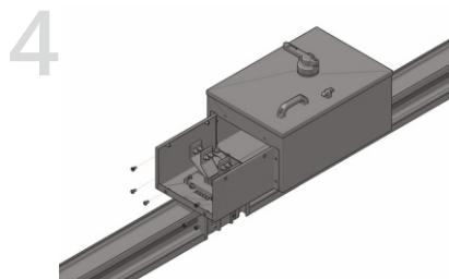
Use M6x12 screws to screw the joint unit and the bolt-on together.
